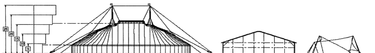
Figure 3 Application of wind load as per EN 13782
